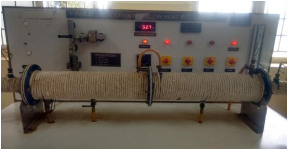
Fig: 1 Experimental setup of tube and tube H.E.
