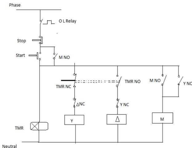
Fig. 2 Control Circuit diagram for Automatic star-delta starter
