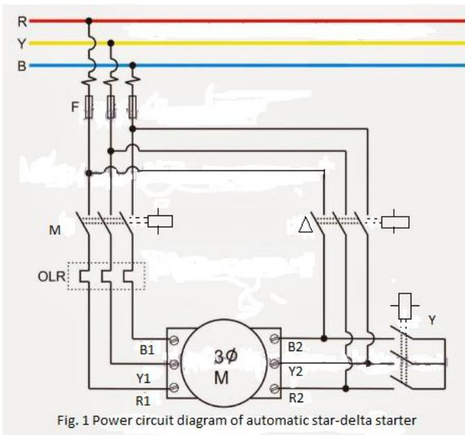
Fig. 1 Power circuit diagram of automatic star-delta starter
