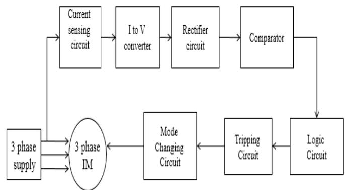
**Fig.3:** Block Diagram of Proposed Starter
