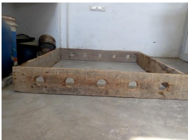
Fig 1: mould of hollow slab
