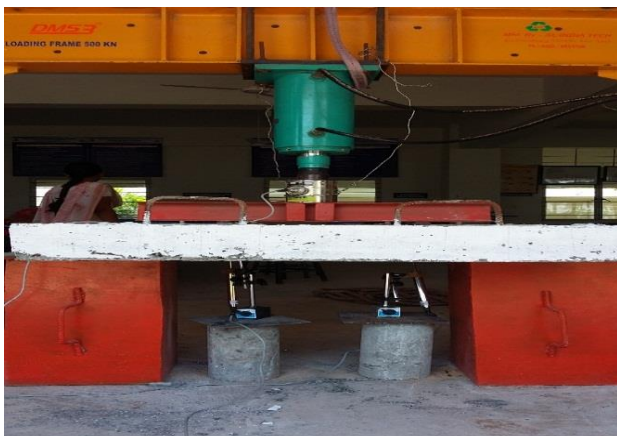
Fig 3: Testing of prestress hollow core slab
