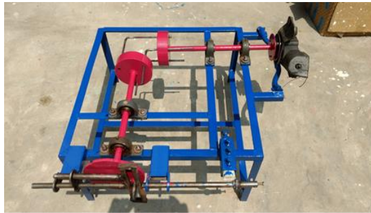
Fig-7: Gearless power transmission for skew shafts
