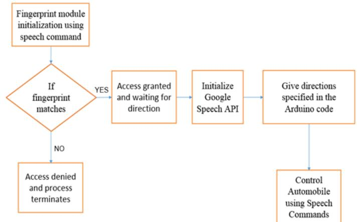
Fig-4: Flowchart of Fingerprint module
