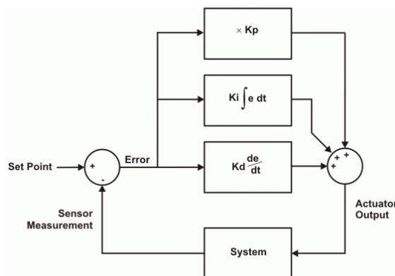
Fig.3 Block diagram of PID controller
