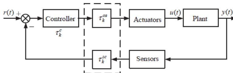
Fig.1. The system block diagram of NCS
