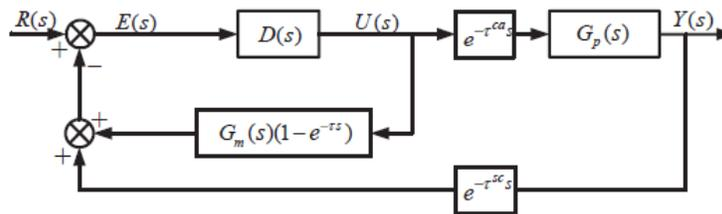
**Fig.5 Block diagram of smith predictor**
