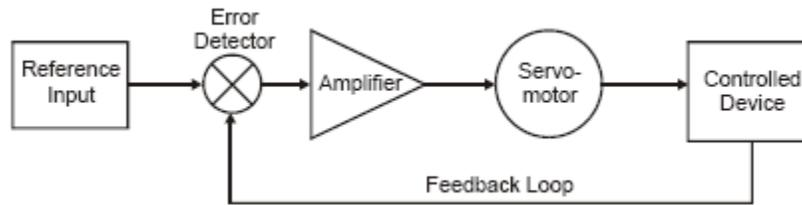
Fig.2. Basic servosystem block diagram
