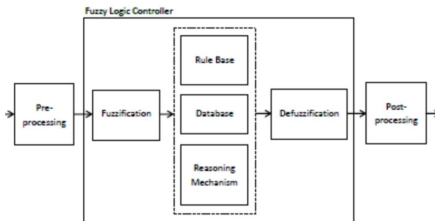
**Fig.4 Fuzzy logic controller structure**
