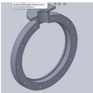
Fig -3(b): Middle Compartment of Annular Casing
