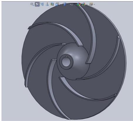
Fig -2: Model of the impeller.
