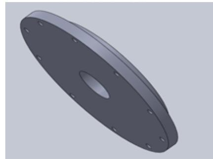
Fig -3(c): Front Compartment of Annular Casing
