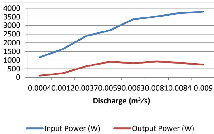
**Chart -2:** Performance Characteristics of Pump at 3mm Tip Clearance
