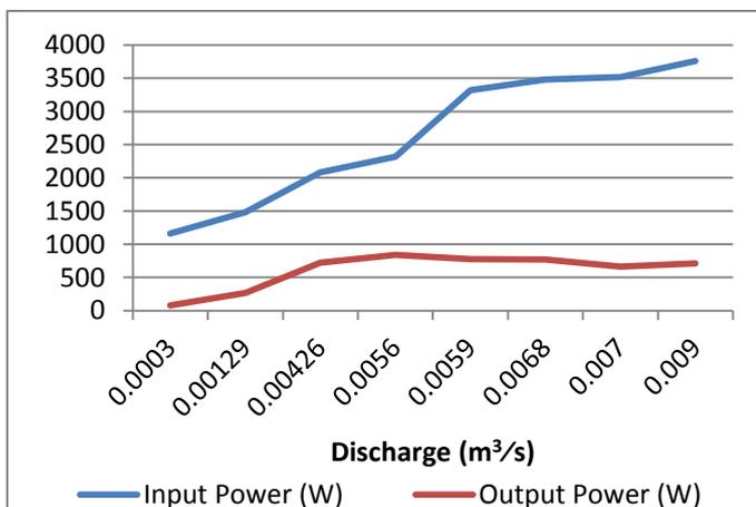
**Chart -3:** Performance Characteristics of Pump at 4.5mm Tip Clearance
