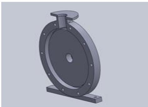
Fig -3(a): Rear Compartment of Annular Casing
