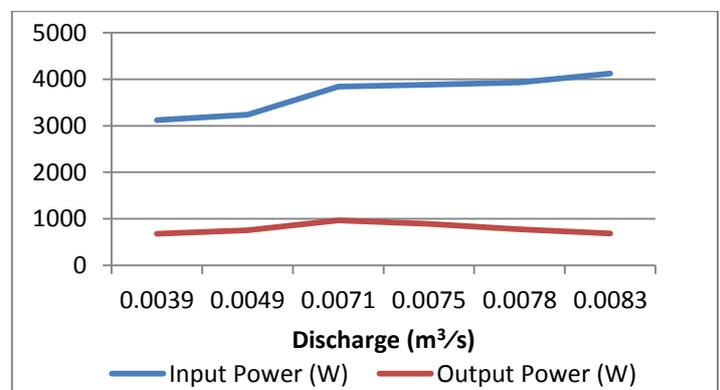
Chart -1: Performance Characteristics of Pump at 1.5mm Tip Clearance
