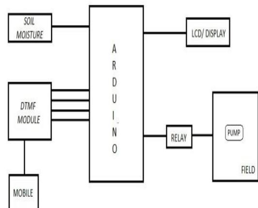
**Fig -1:** Block diagram of module
