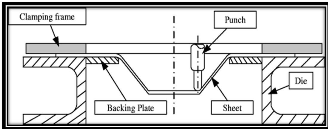
**Fig.1 Single Point Incremental Forming**
