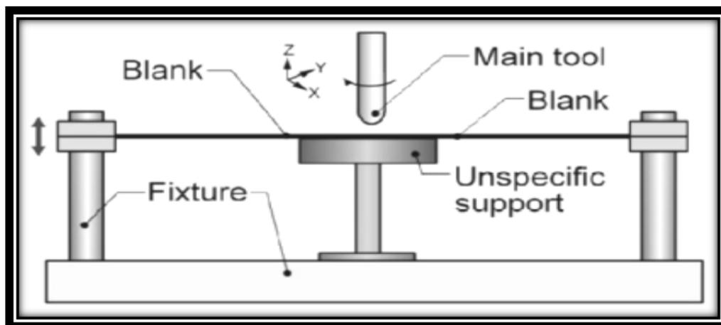
**Fig.2 Two Point Incremental Forming**
