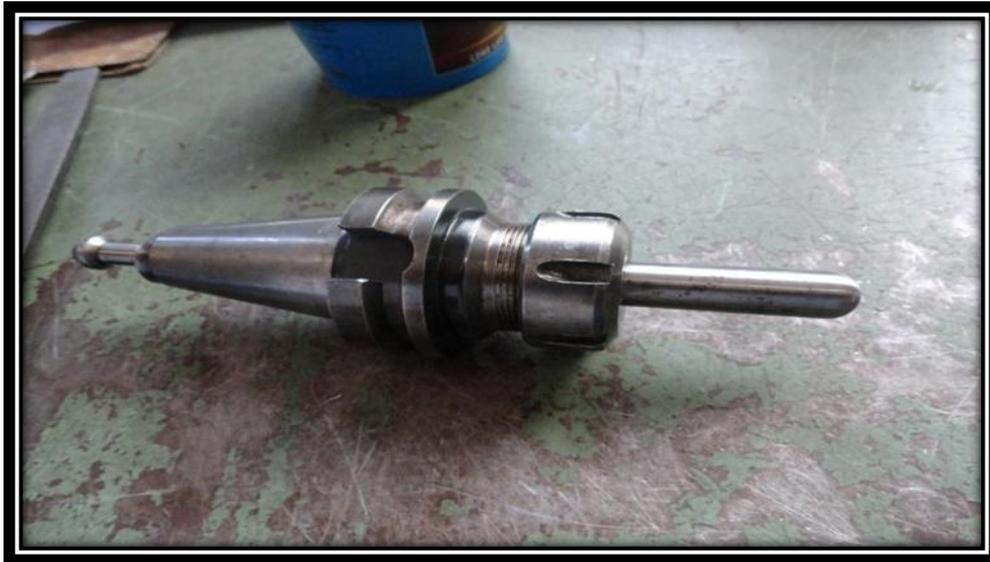
**Fig 3 Stainless Steel Tool of Diameter 16 mm**
