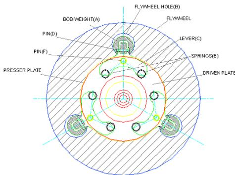
**Fig-4:** Outside End View Of Newton Automatic Centrifugal Clutch
