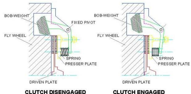
Fig -3: Principle of Newton Automatic Centrifugal Clutch
