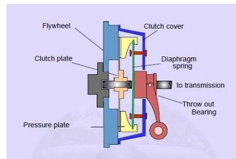
**Fig -1: SINGLE PLATE OR DISC CLUTCH**
