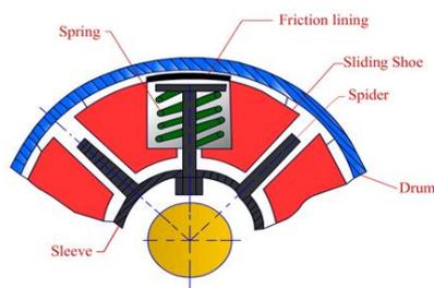
Fig -2: CENTRIFUGAL CLUTCH
