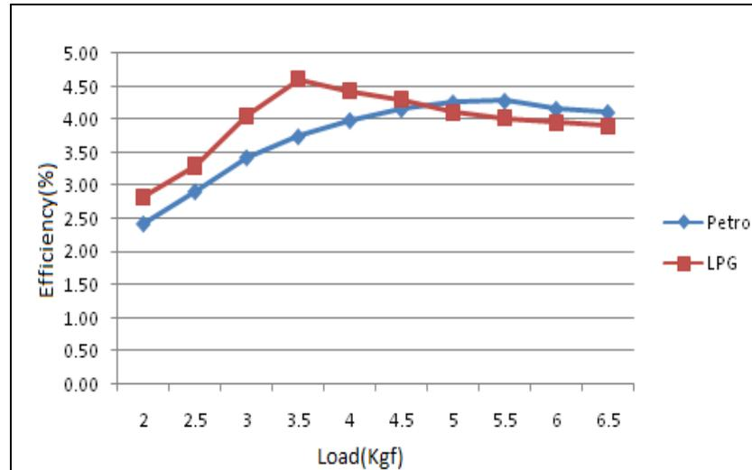
Figure: 5 Load vs brake thermal efficiency
