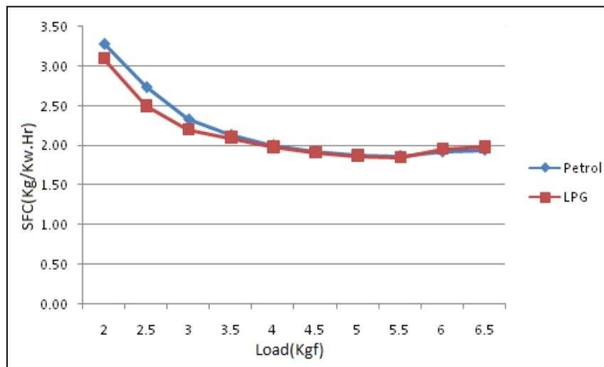
Figure: 4 Load and specific fuel consumption
