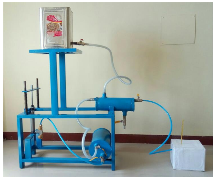
Fig-6: Air cooling system through vehicle suspension
