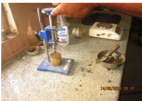
Fig.5 LIQUID LIMIT TEST IN PROGRESS BY CONE PENETROMETER APPARATUS
