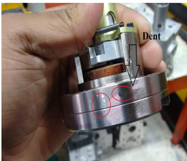
Fig-3: Damaged Actuator
