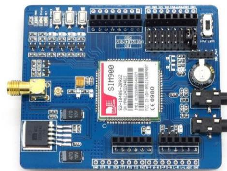
Fig -6: GSM Sim 900
