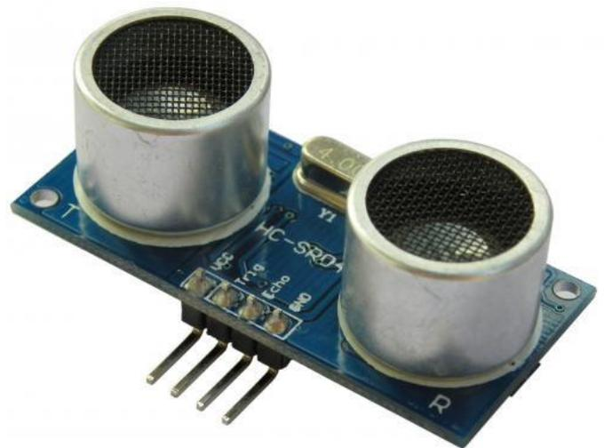
Fig -2: Ultrasonic Sensor
