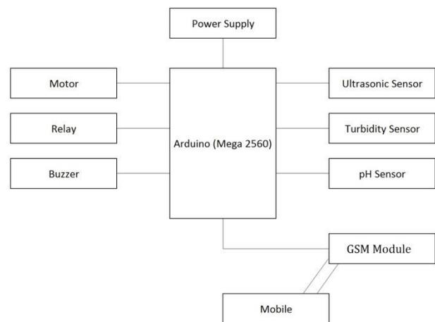
Fig-1 Block diagram of the Chlorine level controller
