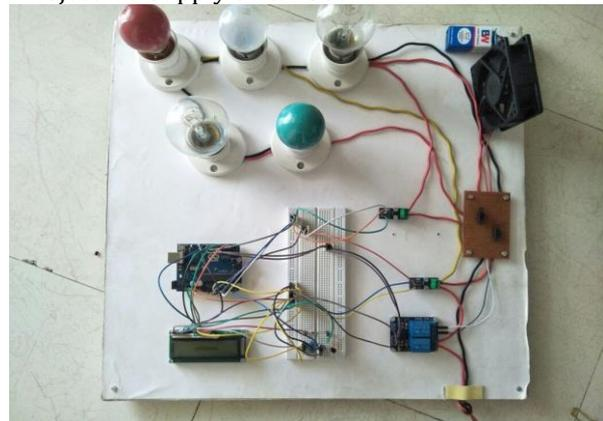
**1) Single phasing fault detection**
