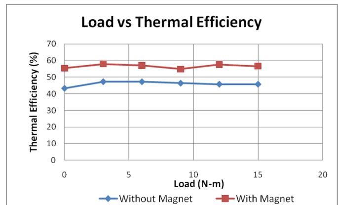
Chart -3: Load vs. Thermal efficiency
