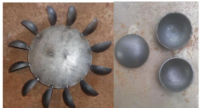
**Fig7: Pelton wheel turbine and cups**
