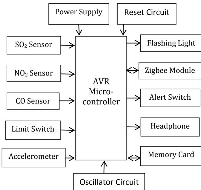
Fig-1: Block diagram of transmitter side of smart helmet
