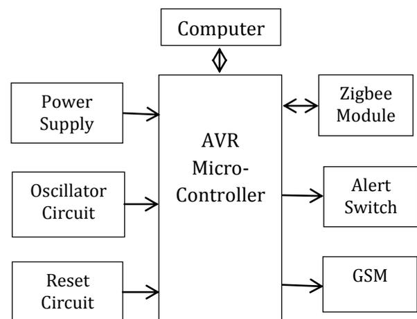
Fig-2: Block diagram of Receiver side of base station
