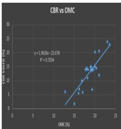
Fig 1: Regression Analysis between CBR and OMC Using SLRA
