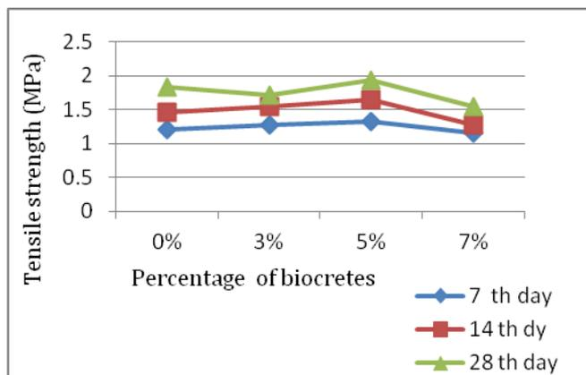
**Chart-2: Split tensile strength for various mix proportions of biocrete at 7<sup>th</sup> and 14<sup>th</sup> and 28<sup>th</sup> day test**
