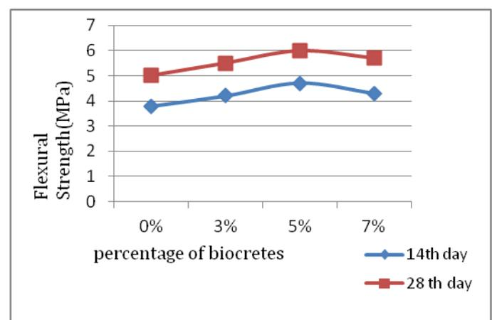
**Chart-5: Flexural strength for various mix proportions of biocrete at 14<sup>th</sup> and 28<sup>th</sup> day test**
