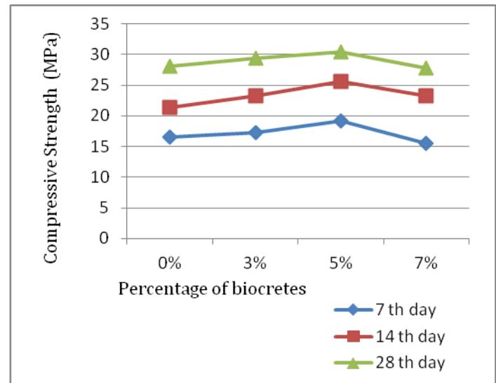
**Chart-1: Compressive strength for various mix proportions of biocretes at 7<sup>th</sup> and 14<sup>th</sup> and 28<sup>th</sup> day test**
