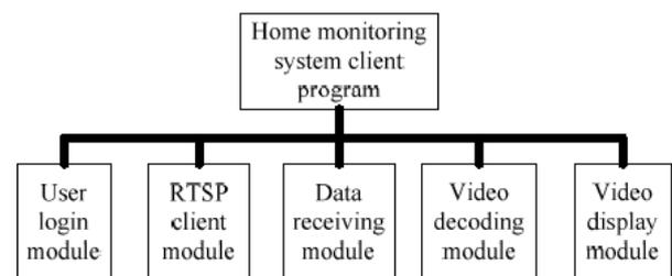
Fig-3: Modules of the monitoring system at the client side.
