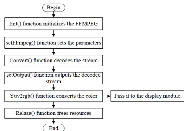
Fig-4: Video decoding process
