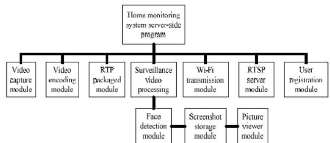
Fig-2: Function structure of the home monitoring at the server side.
