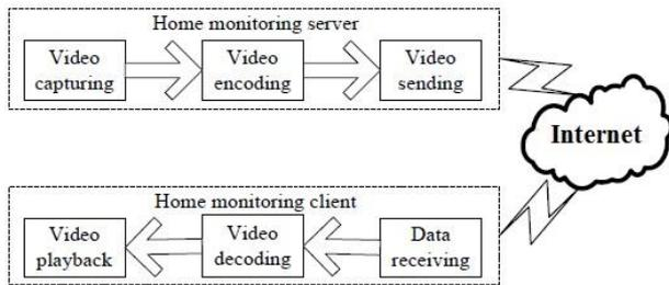
Fig-1: The overall framework of home monitoring system.
