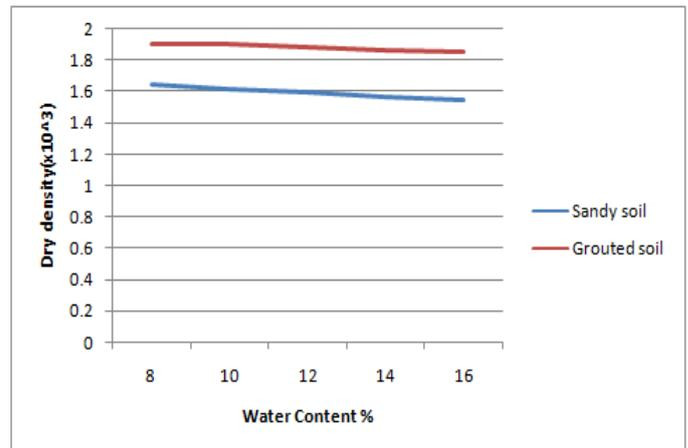
Graph.1. Proctor compaction test values
