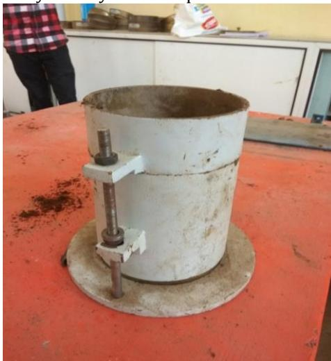
Fig.3. Proctor compaction mould
