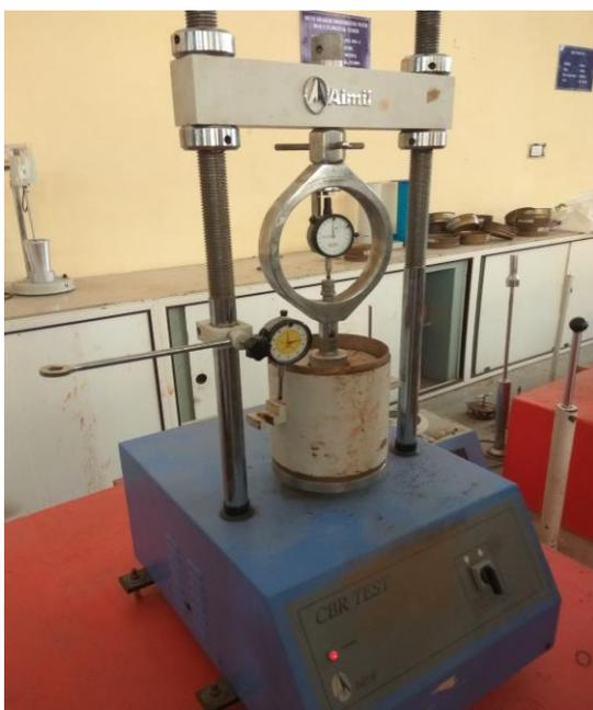
Fig.4. California bearing ratio test
