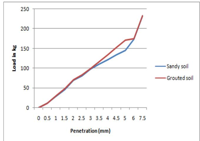
Graph.3. California bearing ratio test value
