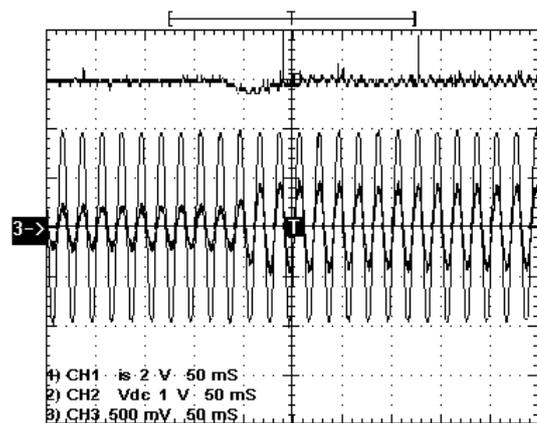
Fig -14: Transient response for a load disturbance.
