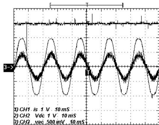
Fig -13: Steady state performance at unity power factor.
