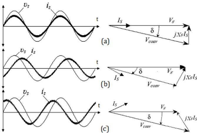
**Fig -6:** Operation of PWM rectifier. (a) operation at unity power factor. (b) operation at leading power factor. (c) operation at lagging power factor.
