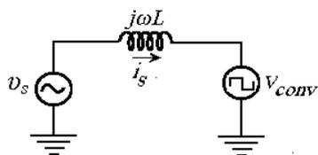
**Fig -4:** Single line representation of the PWM rectifier.
