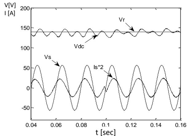
**Fig -9:** Transient response due to lead-lag power factor.
