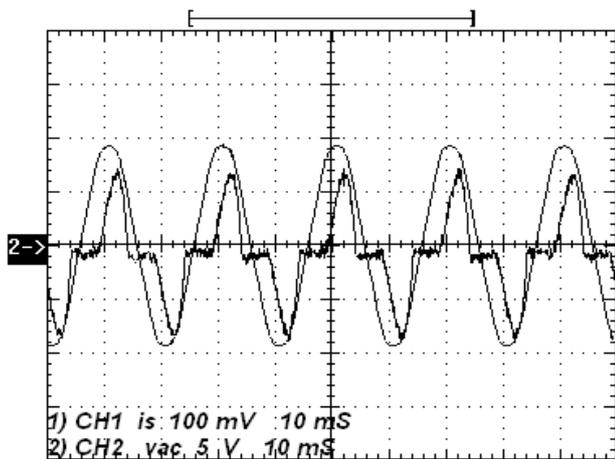
Fig -12: Source current of diode bridge rectifier.
