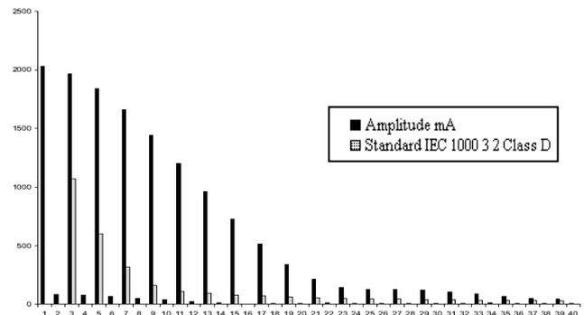
Fig -1: Harmonics spectrum of line current of diode rectifier compared to IEC standard.
