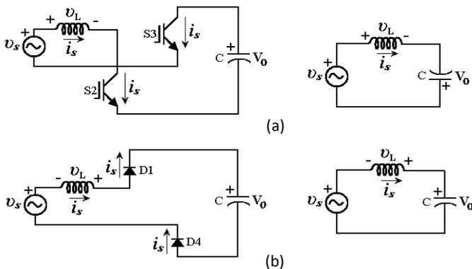
**Fig -3:** Equivalent circuit of PWM rectifier, (a) when S2, S3 ON, (b) when S2, S3 OFF.
