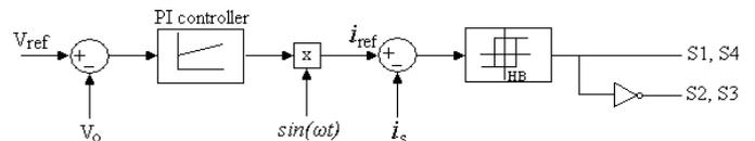
**Fig -5:** Block diagram of implemented control strategy.
