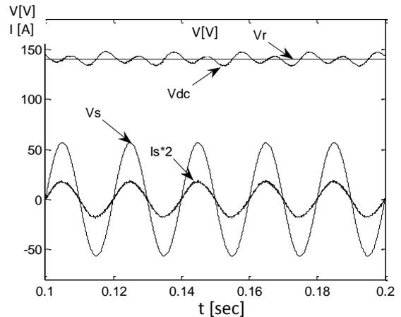
**Fig -8:** Steady state performance at unity power factor.
