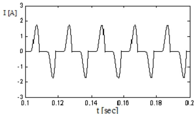
**Fig -7:** AC line current of diode rectifier
