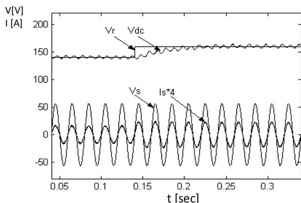
**Fig -10:** Transient response due to step change in reference load voltage.
