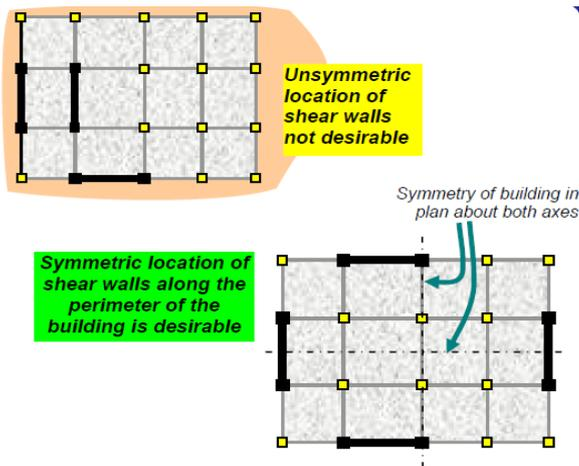
**Fig 2 Location of shear wall**
