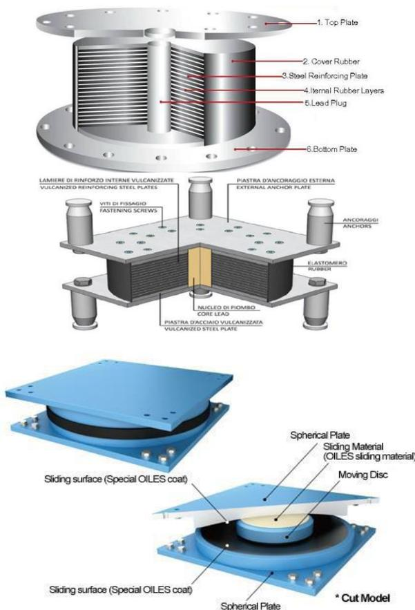
Fig. 1 Elastomeric systems and Sliding Type Base Isolator
