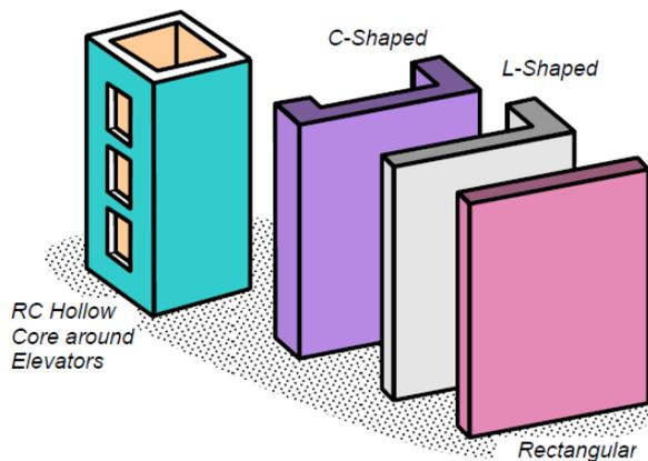
**Fig 3 Different geometries of shear wall**
