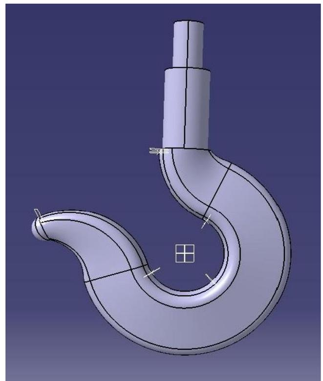
Fig 1.1 Solid Modelling of Crane Hook
