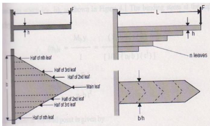
**Fig-2-** Leaf spring representation as triangular plate [7]
