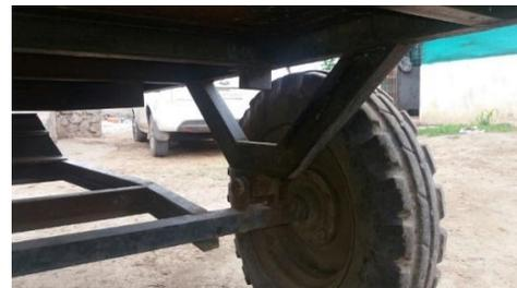
**Fig-1-** Rigid joint of agricultural trolley
