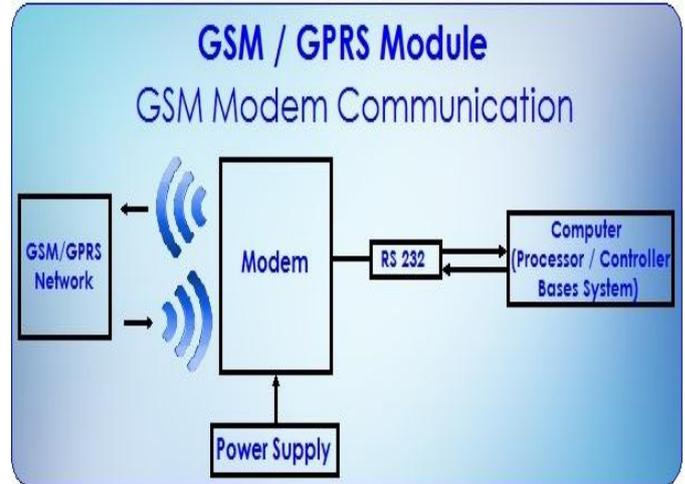
Fig-2: GSM Modem Communication
