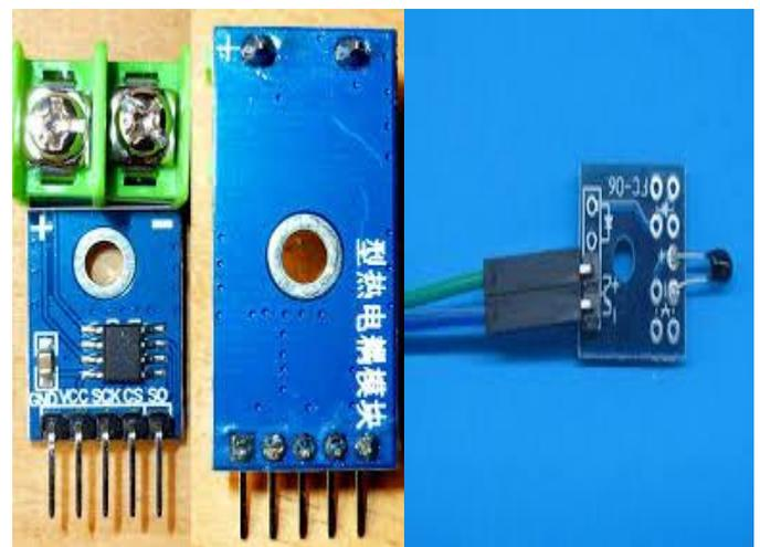
**Fig-6:** Temperature Sensor
