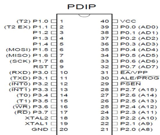
Fig -3: Pin Configuration of Microcontroller
