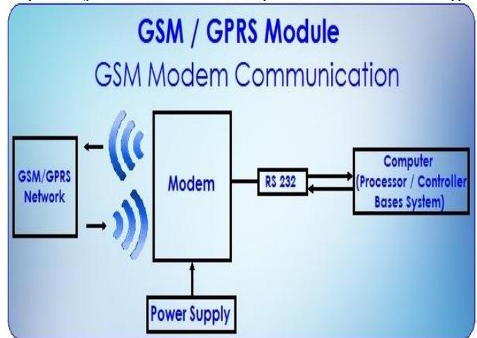
Fig-2: GSM Modem Communication
