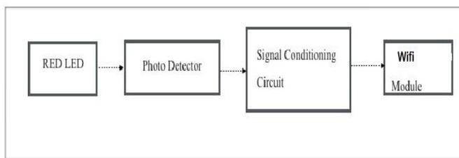
**Fig-4:** Block Diagram of Pulse Rate
