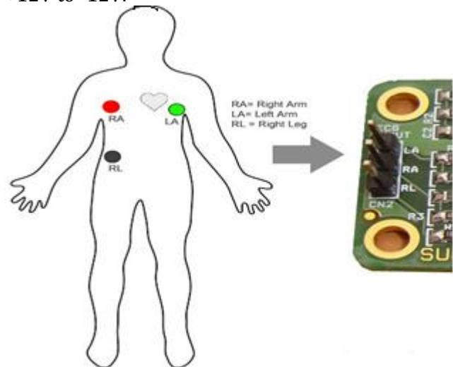
**Fig-5:** Connection for the ECG Sensor
