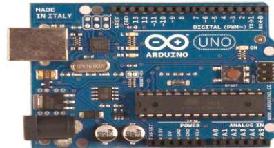
The Arduino Uno is a microcontroller based on the ATmega328. Which having 14 digital input/output pins out of which 6 can be used as PWM outputs,6 analog inputs and a 16 MHz crystal oscillator, a USB connection, a power jack, a ICSP header, and a reset button. It contains everything which is needed to support the microcontroller. The Arduino Uno differs from all preceding boards in that it does not use the FTDI.
