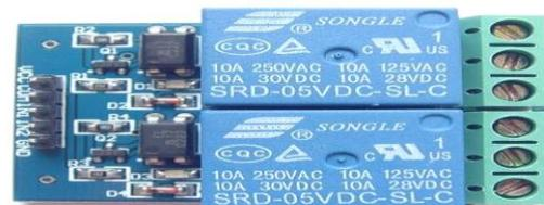
Relay module is an electrically operated switch that allows to turn on or off a circuit using voltage and/or current which is much higher than a microcontroller could handle. There is no connection established between the low voltage circuit operated by the microcontroller and also high power circuit. In this module each channel has three connections named NC (normally closed), NO (normally open) and COM (common).
