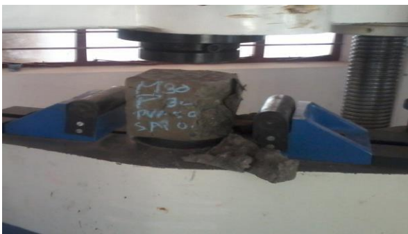
Fig -1: Cube Specimen under Compression Test
