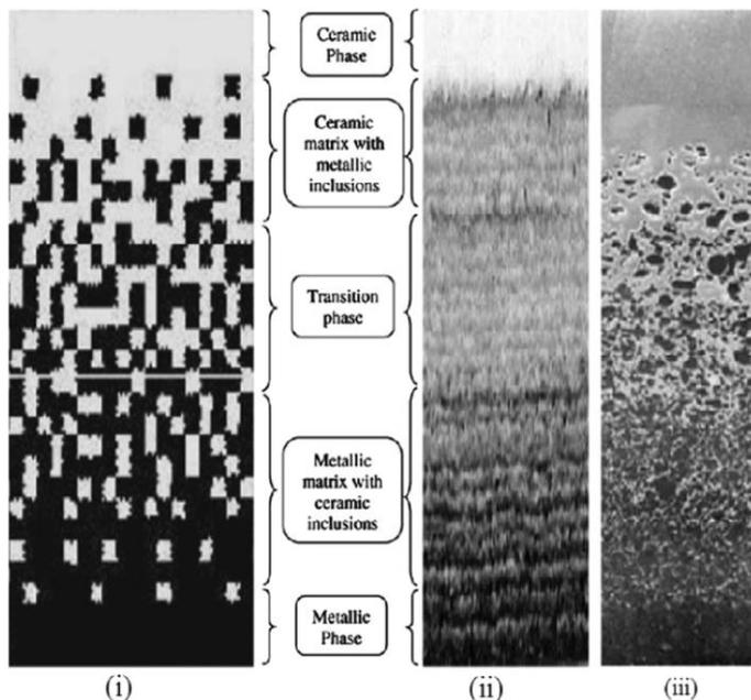
Fig.3. Gradation of microstructure with metal-ceramic constituents: (i) smoothly graded microstructure, (ii) enlarged view and (iii) ceramic-metal FGM
