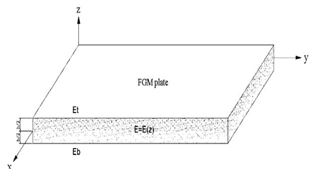
Fig.4. FGM geometry
