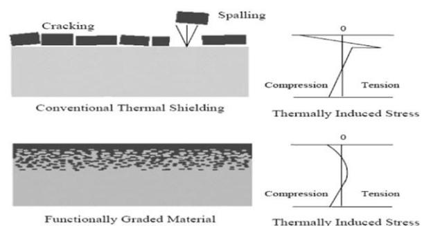
**Fig.1.** Thermal protection of conventional material and FGM
