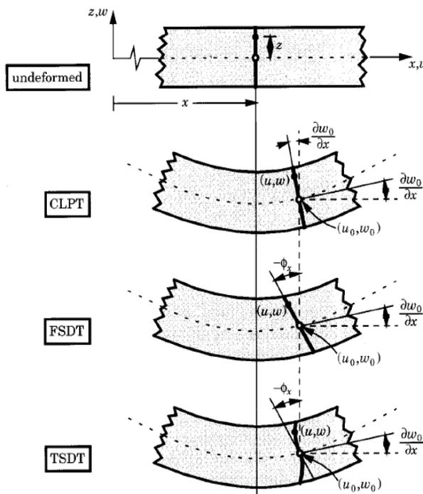
Fig.5. Transverse shear deformation of a plane according to various plate theories
