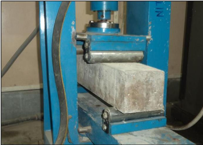
FIG.2. Test for flexural strength of Concrete
