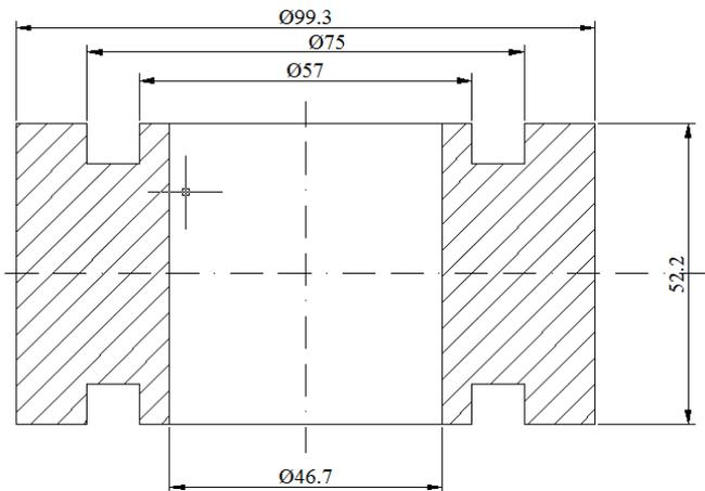
Fig -1: Machining Drawing
