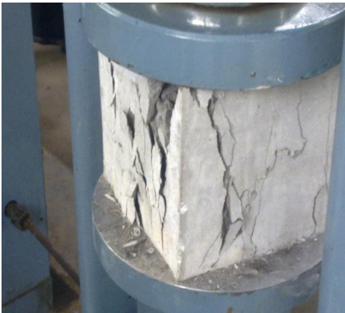
Fig -1: Testing of cube
