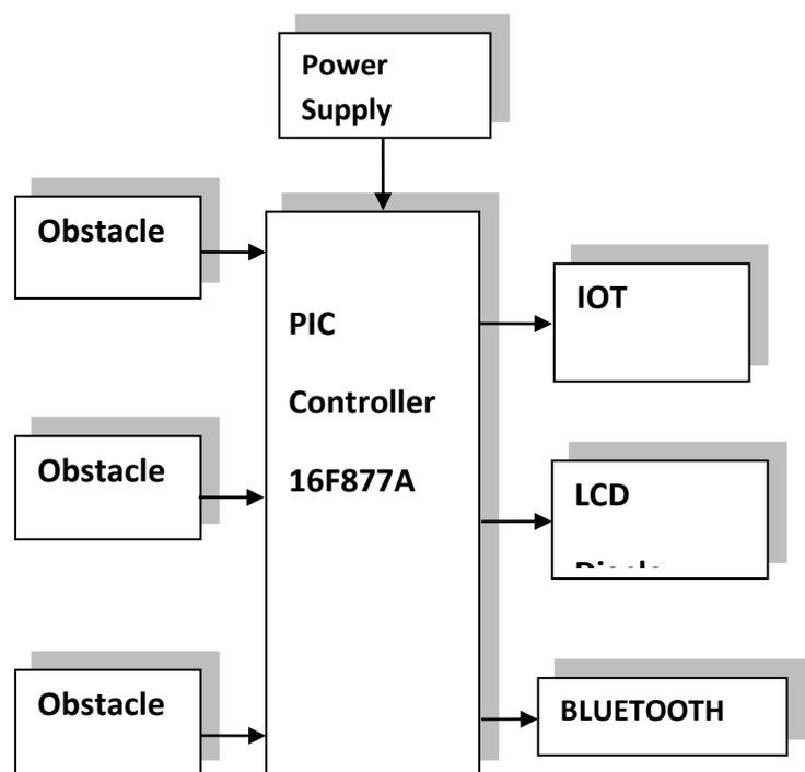
Fig -1: Block diagram of parking system
