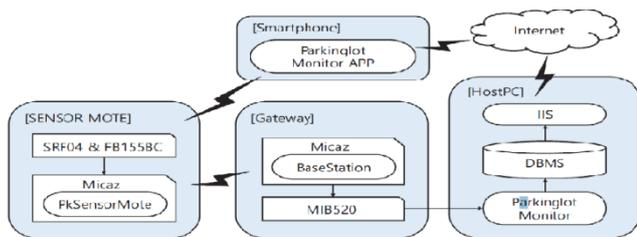
Fig. 3. Software architecture.
