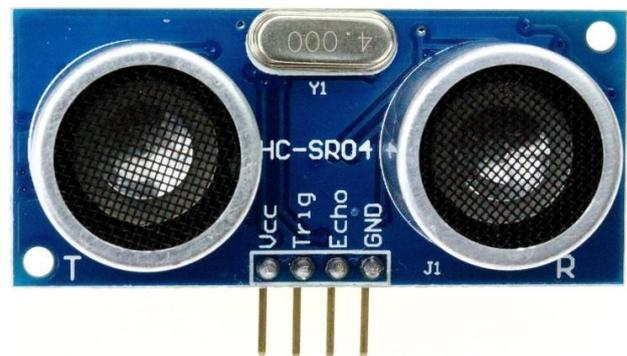
Fig. 2. Ultrasonic sensor
