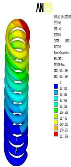
Fig - 4: Displacement z-direction
