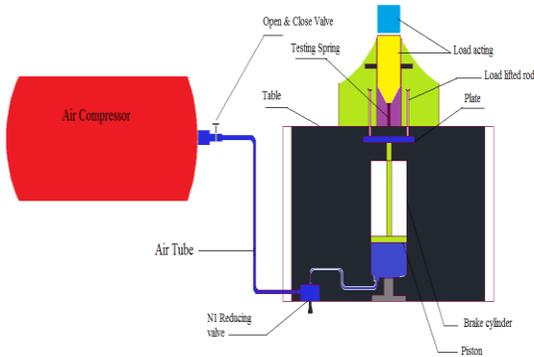
Load testing Machine Layout Diagram
