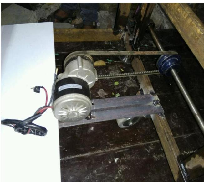
**Fig BELT DRIVE MSM WITH PULLEY.**
