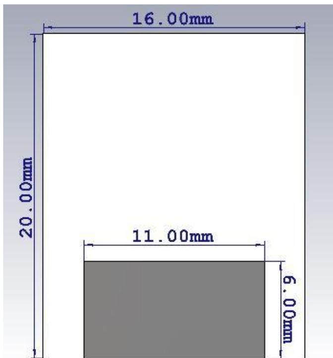
Fig -3: Back view of the proposed antenna
