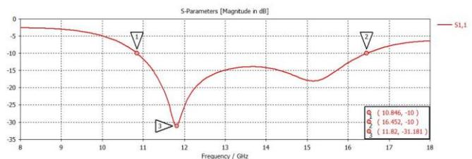
Fig -5: Bandwidth plot of the proposed antenna
