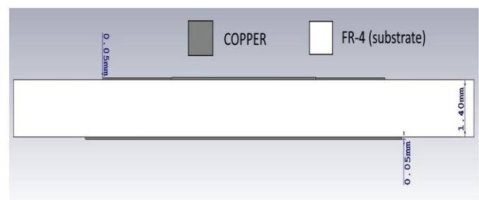
Fig -1: Side view of the proposed antenna
