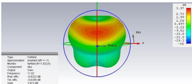
Fig -8: Gain of the proposed antenna
