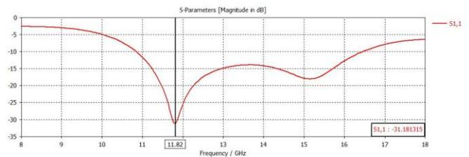
Fig -4: Return loss plot of the proposed antenna
