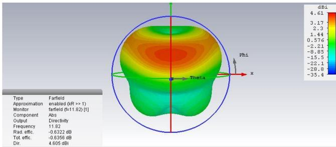
Fig -7: Directivity of the proposed antenna
