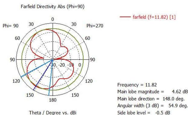
Fig -10: Polar plot of the proposed antenna
