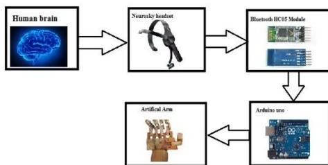
**Fig -1:** Basic block diagram of Brainwave Controlled Robotic Arm.
