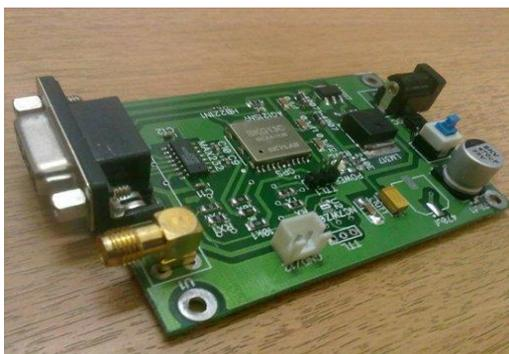
With a tiny configuration of 24mm x 24mm x 3 mm, SIM900 can fit almost all the space requirements in your M2M application, especially for slim and compact demand of design.
