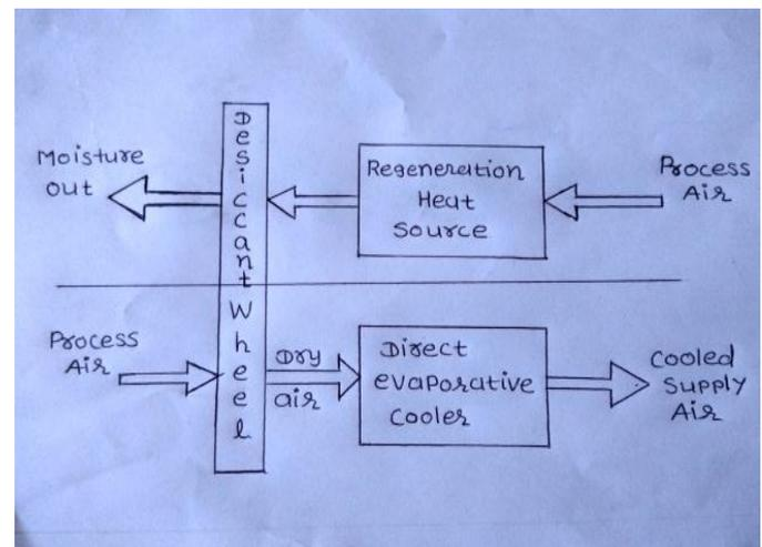
Fig -1: Schematic diagram of the system
