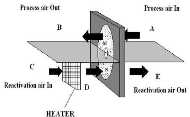
Fig -2: Working of solid desiccant Air conditioning<sup>[2]</sup>
