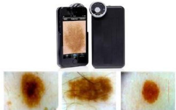
FIGURE 2. The dermoscopy device attached to the iPhone and sample of images captured using the device.
