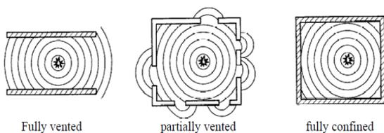
Fig. 3 - Fully vented, partially vented and fully confined explosions
