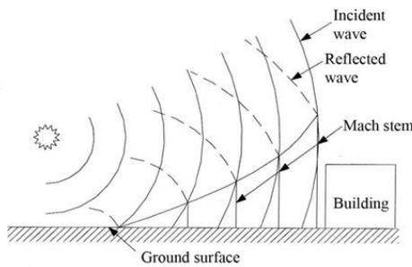
Fig. 1 - Air burst with ground reflections
