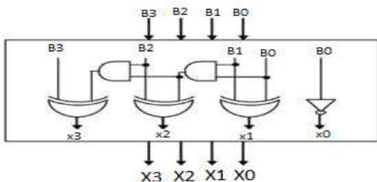
Fig 3.2 : four-bit BEC
