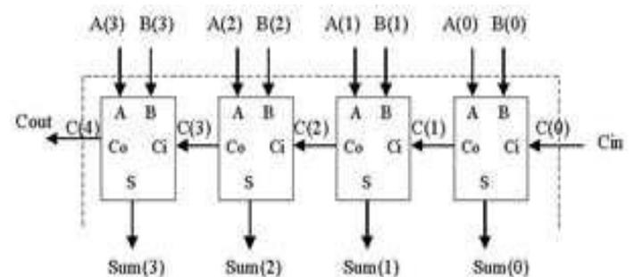
Fig 3.1 : four-bit ripple carry adder
