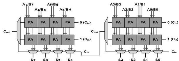
Fig-3.4: block diagram of linear 8 bit CSA
