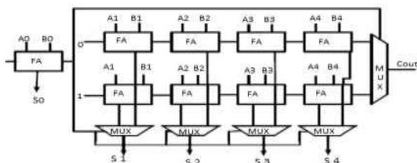
Fig 3.3: Block Diagram of Conventional CSLA
