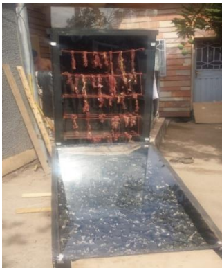
Fig -3: The prototype dryer loaded with meat strips
