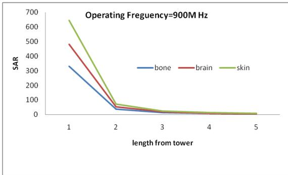
Figure 2: Variation of SAR Vs length of the tower (Meters) at 900MHz.
