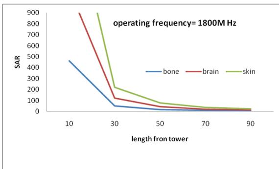
Figure 3: Variation of SAR Vs length of the tower (Meters) at 1800MHz.
