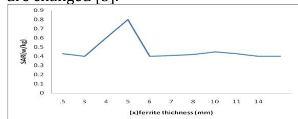
Figure 4: SAR vs Ferrite thickness
