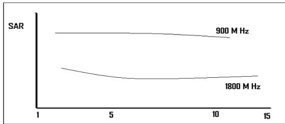
Figure 7: Distance from the Head to Mobile Phone
