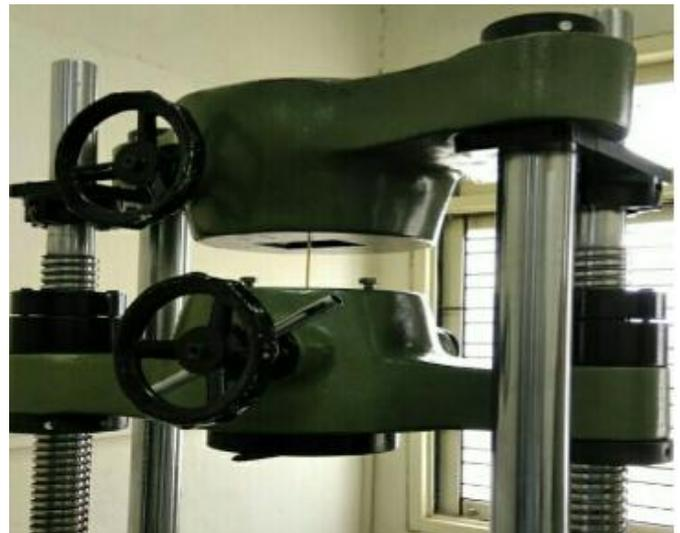
Figure 8. Breaking load test in UTM
