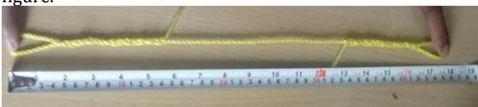
Figure 7. Sample of 450mm in length with splice
