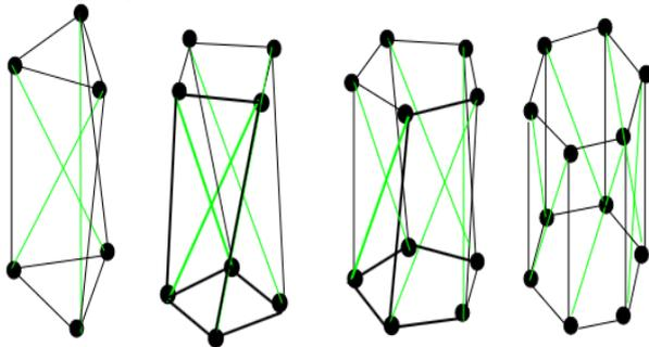
Figure 3. Class-I tensegrity 3D prism [2]
