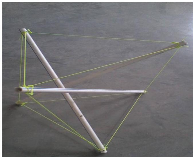
Figure 4. Tensegrity 3-strut model
