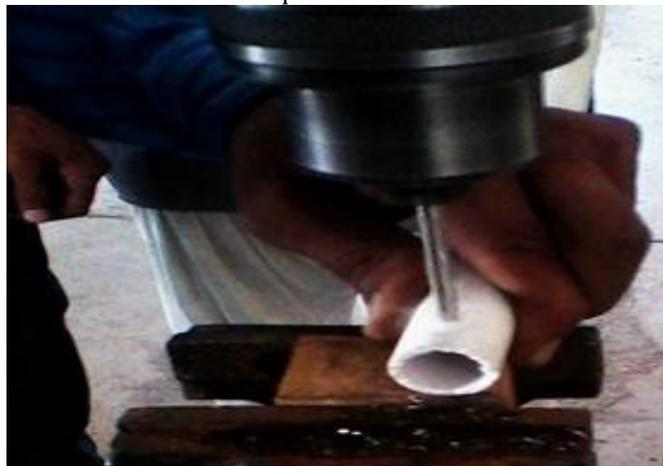
Figure 11. 10mm hole at the ends of UPVC Pipe
