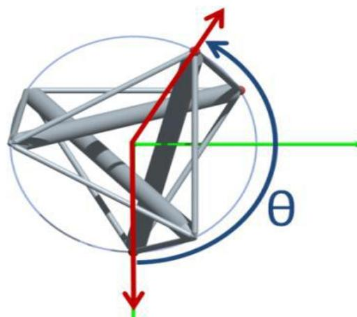
Figure 9. Strut angle [13]
