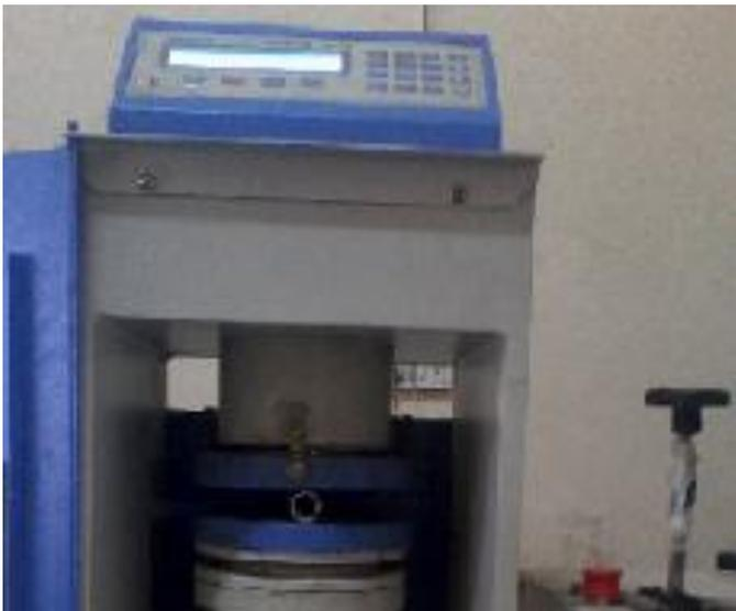
Figure 6. Parallel Plate Loading test (stiffness test)
