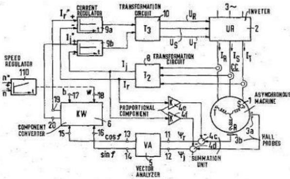
Fig-1: Block diagram from Blaschke's 1971 US patent application
