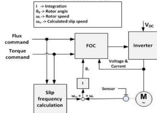
Fig-7: Simplified Indirect FOC Block Diagram
