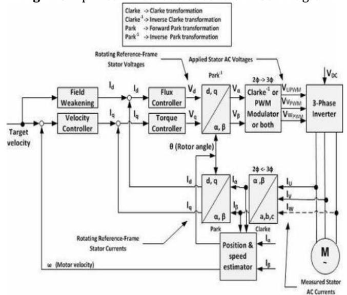
Fig-5: Vector control Block Diagram
