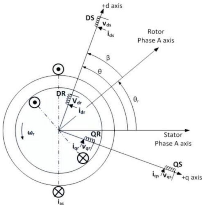
Fig-6: (D-Q) Coordinate System Superimposed on Three-Phase Induction Motor
