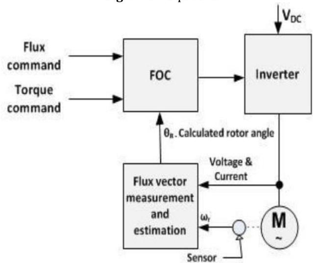
Fig-4: Simplified Direct vector control Block Diagram
