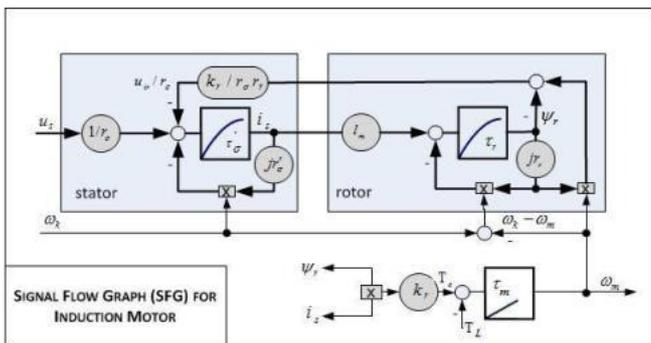
Fig-2: Signal Flow Graph (SFG) for Induction Motor
