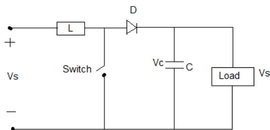
Fig. 3: Boost converter Configuration
