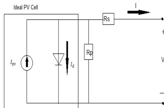
Fig. 2: PV cell single diode model
