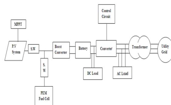
**Fig.1.** Components of Grid connected PV plant
