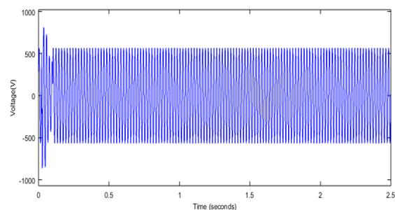
Fig. 17: Grid side voltage of main converter
