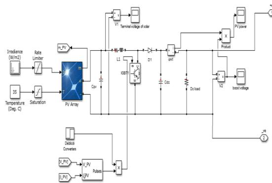
Fig. 7: Simulation of PV Array and Boost Converter
