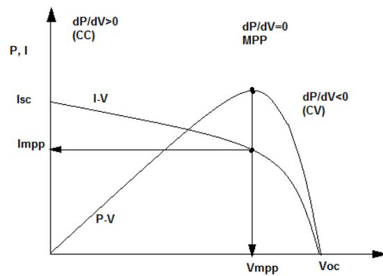
Fig. 4:  $I$ - $V$  and  $P$ - $V$  characteristics of PV array
