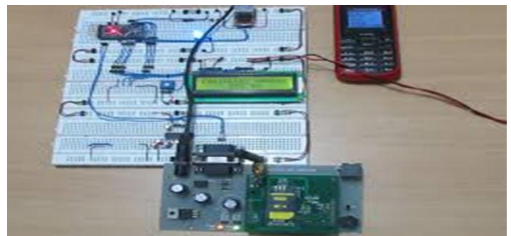
Fig 1, shows the image after implementation which consists of gas sensor, LCD display, GSM.
